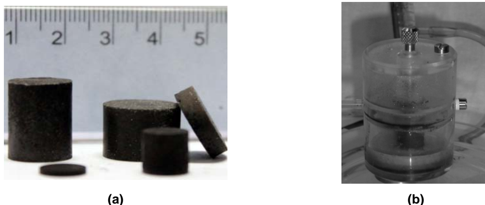
Fig. 1. (a) «Hydrogen pellets» based on NaBH 4 and (b) hydrogen generator
